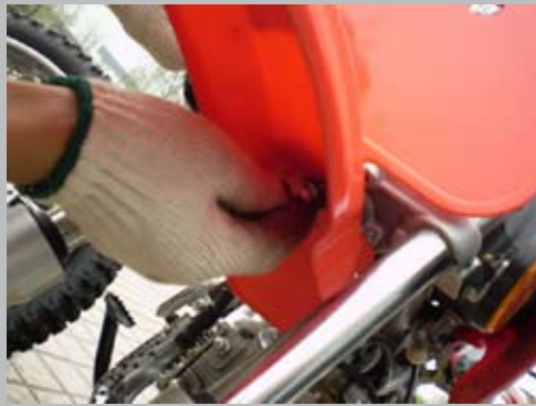
Using the third screw to fix the front fender and No. plate.
